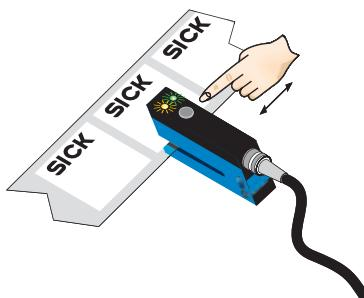
Press the teach-in button for 3 - 20 s. With the pushbutton pressed down, move several label with carrier material (label) through the sensor. The yellow LED flashes at 3 Hz during the teach-in procedure. Recommendation: Move at least 3 label + carrier through the sensor.
