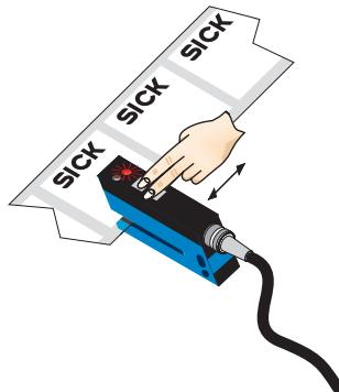
Press both the “+” and “-” buttons together, hold > 1 s and then release the teach-in buttons. The red LED flashes.
