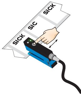
Press the teach-in button for 3 - 20 s. With the pushbutton pressed down, move several label with carrier material (label) through the sensor. The yellow LED flashes at 3 Hz during the teach-in procedure. Recommendation: Move at least 3 label + carrier through the sensor.
