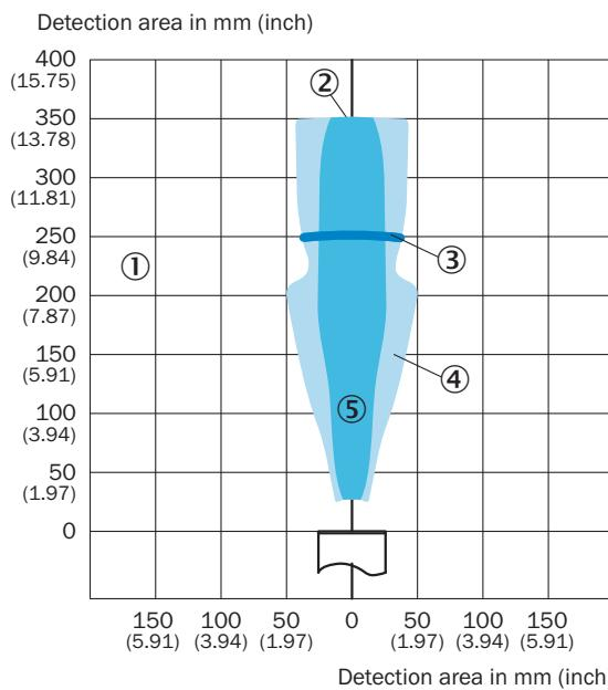
① Detection range dependent on reflection properties, size, and alignment of the object
