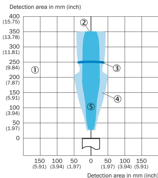
① Detection range dependent on reflection properties, size, and alignment of the object
