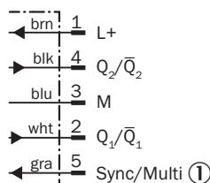
① Synchronization and multiplex mode, Connect+ communication
