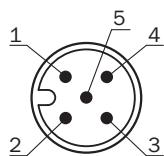
Connection diagram UM30-21x112 UM30-21x115 Connector M12, 5-pin
