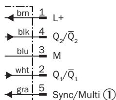
① Synchronization and multiplex mode, Connect+ communication
