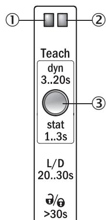
① Function signal indicator (yellow), switching output
