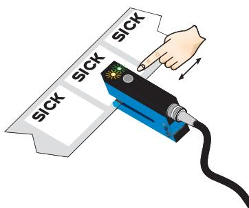
Release the teach-in button for < 20 s. If teach-in is successful, the function indicator (yellow LED) directly indicates the output state of the sensor. The switching threshold is now optimally set between carrier and label. The best possible operational safety is provided.
