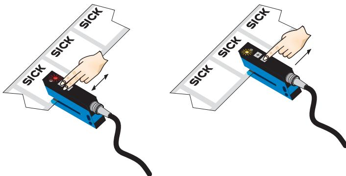
Press both the “+” and “-” buttons together, hold > 1 s and then release the teach-in buttons. The red LED flashes.
