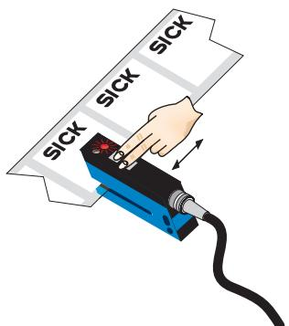
Press both the "+" and “-” buttons together, hold > 1 s and then release the teach-in buttons. The red LED flashes.
