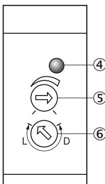
④ Orange LED indicator : switching output active
