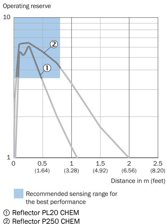
Characteristic curve Fine triple reflectors
