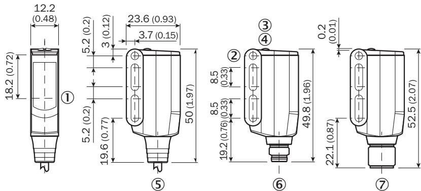
① Sender and receiver optical axis center
