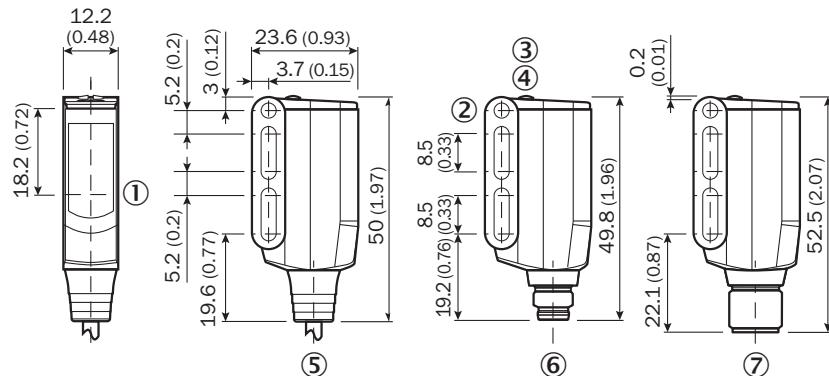
① Sender and receiver optical axis center
