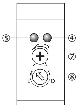
④ Orange LED indicator : switching output active
