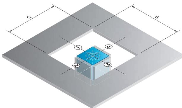
Sensor with rotated turning angle (the specified values refer to 1 mm thick sheet steel).
