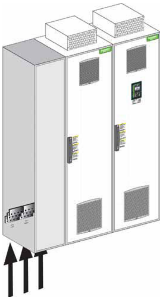
Additional enclosure allowing cabling from the bottom
