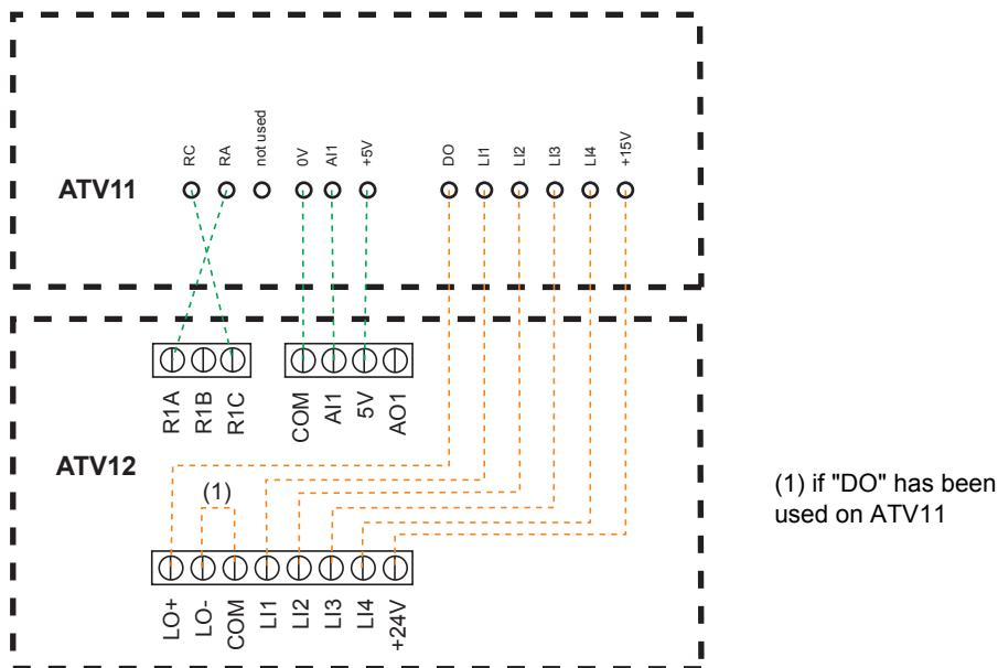
(1) On ATV11 DO is an analog output that can be configured as a logic output. On ATV12, depending on your configuration, DO can be linked to LO1 or AO1.
