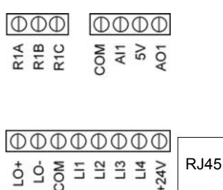
Note: To connect cables, use a slotted screwdriver 0.6 x 3.5.
