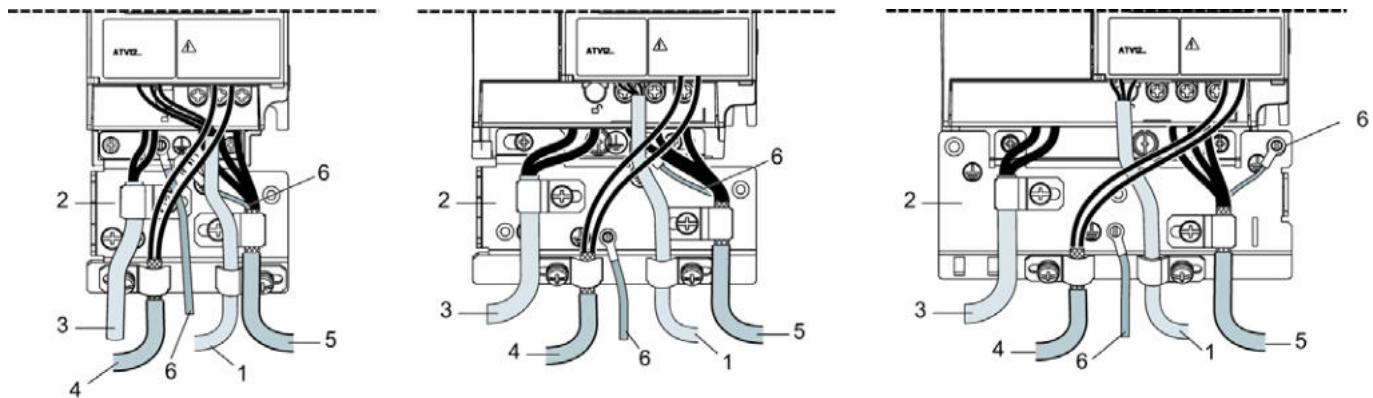
1. Non-shielded wires for the output of the status relay contacts.
