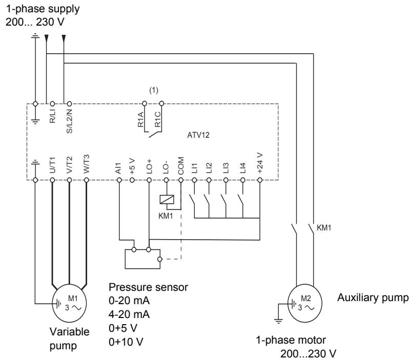
(1) Fault relay contacts, for remote indication of the drive status.
