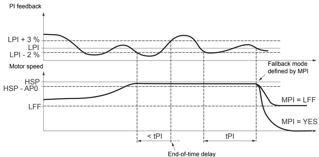
Once the variable pump is running at maximum speed (higher than HSP - AP0) and at the same time the PI feedback is lower than the supervision threshold LPI - 2%, a time delay  $tPI$  is launched. If at the end of this time delay the value of the PI feedback is still lower than the supervision threshold LPI + 3%, the drive switches to fallback mode as defined by parameter MPI.
