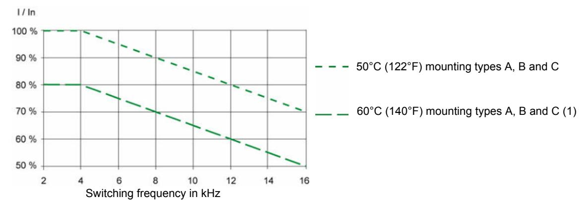
For intermediate temperatures (for example 55°C (131°F)), interpolate between 2 curves.
