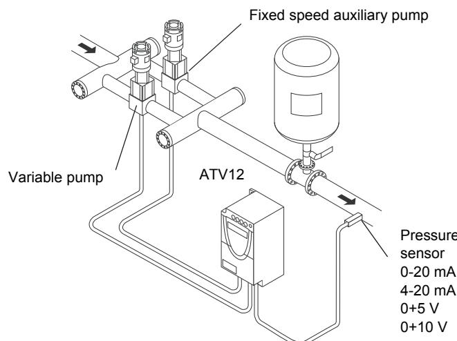
The auxiliary pump is controlled by the Altivar 12 via logic output LO.
