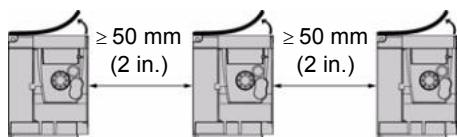
Free space  $\geq 50$  mm (2 in.) on each side. Vent cover should be removed for operation at surrounding air temperature above 50°C (122°F).
