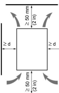
Install the unit vertically, at  $\pm 10^\circ$ .
