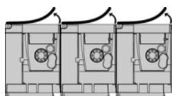
Drives mounted side-by-side, vent cover should be removed.
