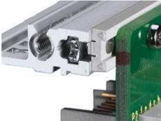
Indirect backplane mounting (with insulation strip)
