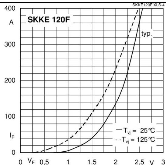
Fig. 4 Typ. forward characteristics
