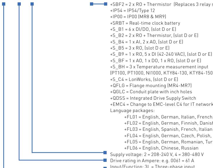
Standard delivery includes IP21/ Type 1, EMC level C2, graphical display keypad, relay board 1 +SBF1 (3 x RO) and +FL01.
