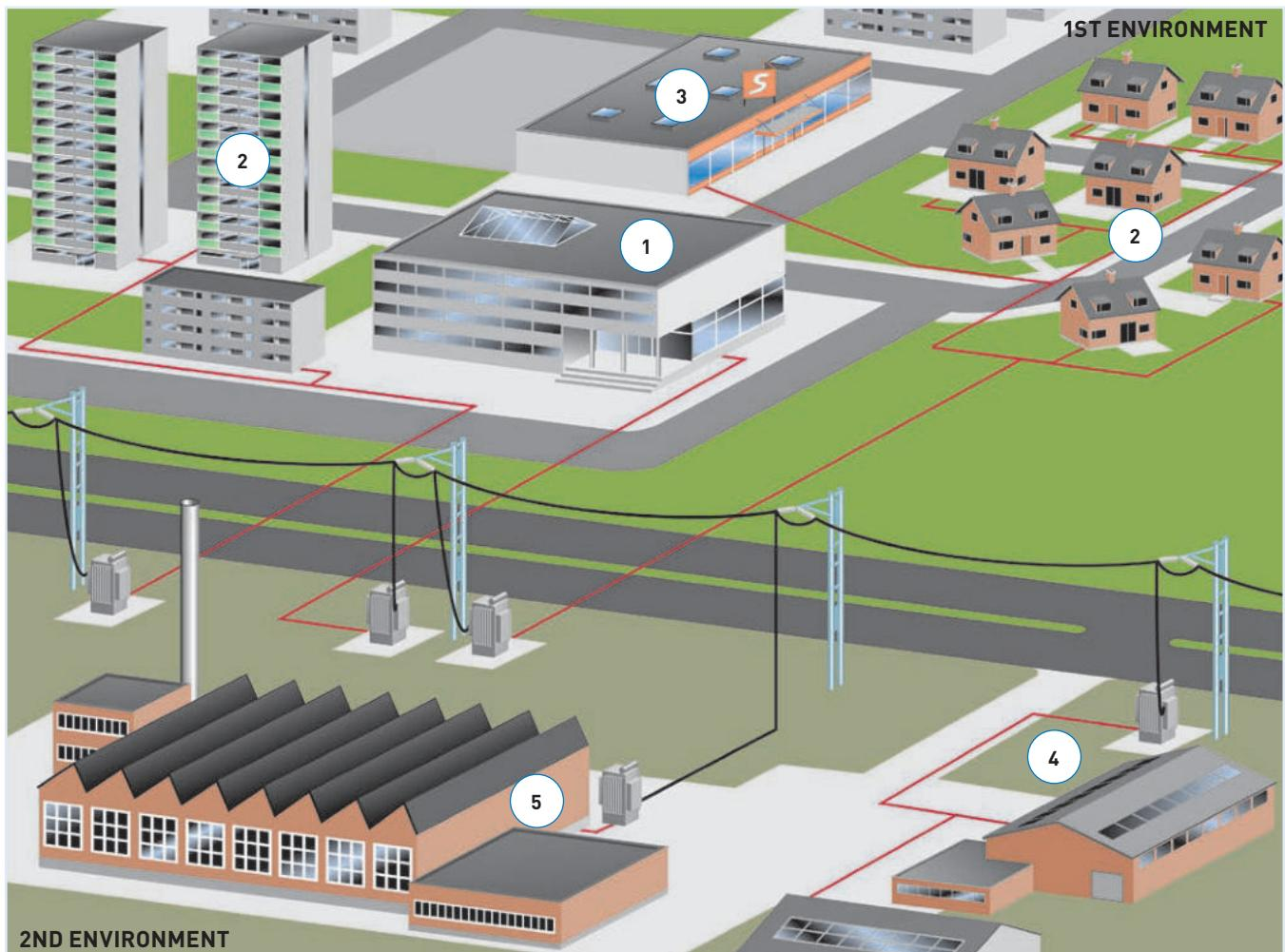
The product family standard EN61800-3 sets limits for both emissions and immunity of radio frequency disturbances. The environment has been divided into the 1st and 2nd environments, which, in practice, means public and industrial networks.
