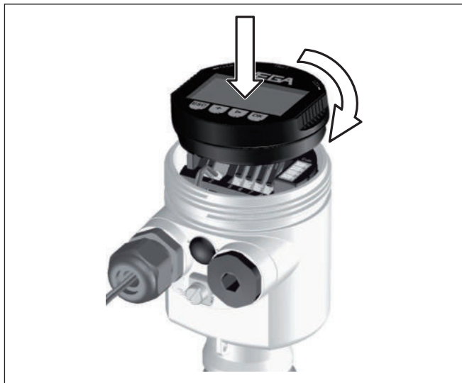
Fig. 29: Insert display and adjustment module in the single chamber housing
