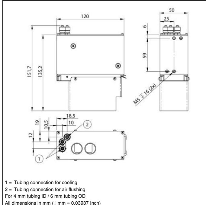
1 = Tubing connection for cooling
