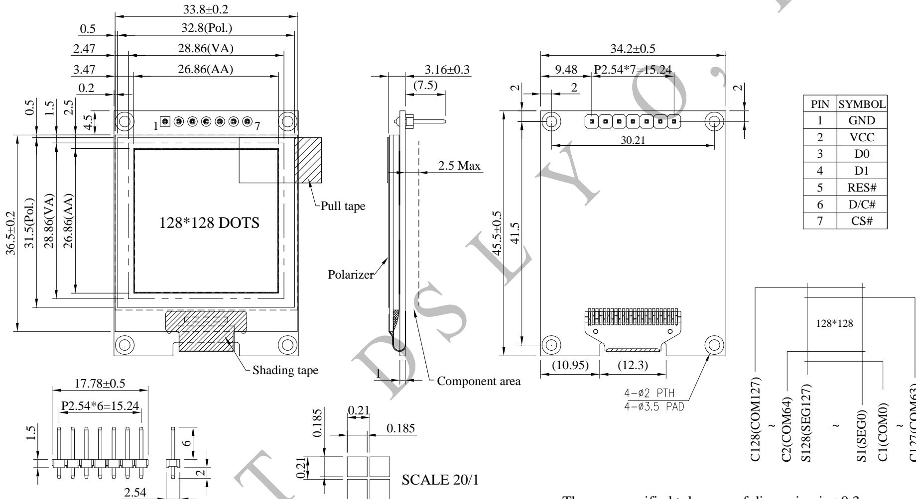
The non-specified tolerance of dimension is  $\pm 0.3$  mm .
