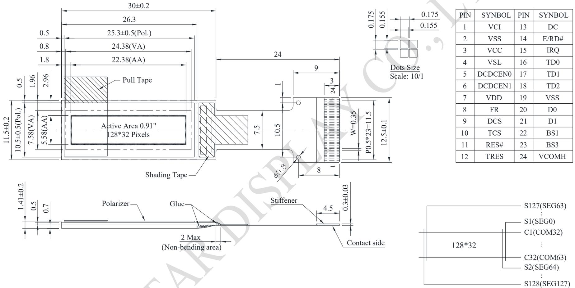
The non-specified tolerance of dimension is  $\pm 0.3$  mm .
