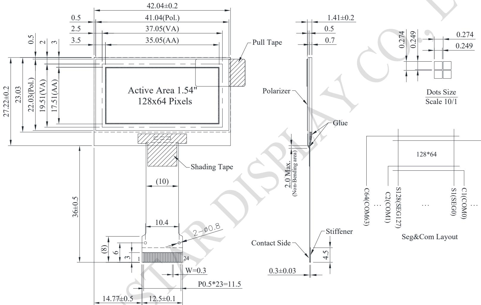
The non-specified tolerance of dimension is ±0.3 mm .
