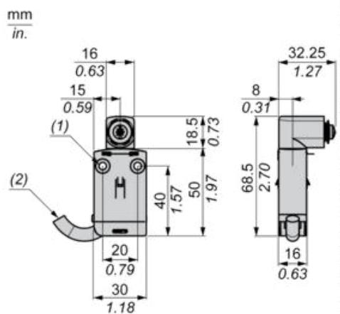
(1) 2 fixing holes Ø 4.2 mm, counterbored Ø 8 mm by 4 mm deep.
