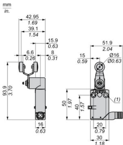
(1) 2 fixing holes Ø 4.2 mm, counterbored Ø 8 mm by 4 mm deep.
