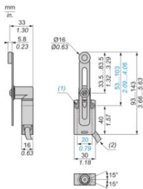
(1) 2 fixing holes Ø 4.2 mm, counterbored Ø 8 mm by 4 mm deep.
