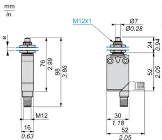
e : 8 mm max, panel cut-out Ø 12.5 mm, fixing nut thickness 3.5 mm.
