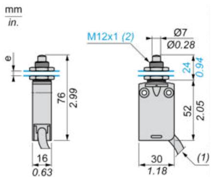
(1) External diameter of cable 7.5 mm.
