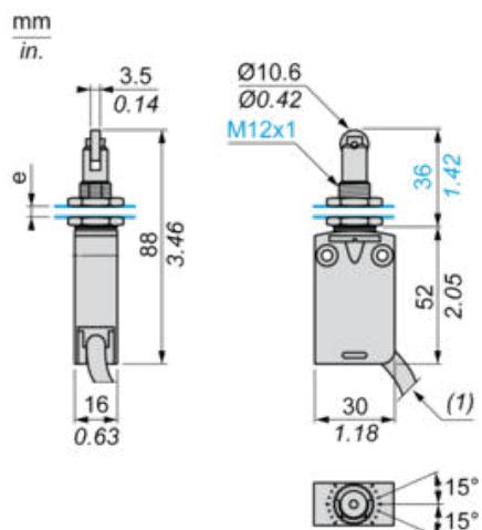
(1) External diameter of cable 7.5 mm.
