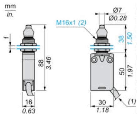
(1) External diameter of cable 7.5 mm.
