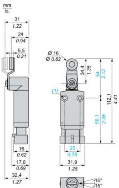
(1) : 2 fixing holes Ø 4.2 mm, counterbored Ø 8 mm by 4 mm deep.
