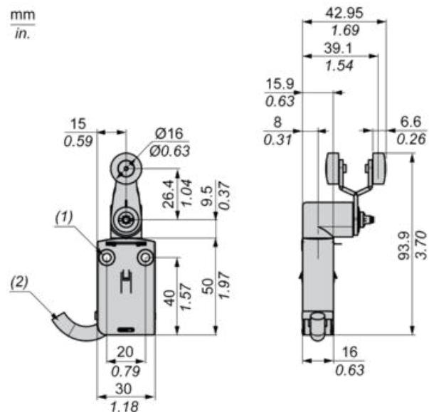
(1) 2 fixing holes Ø 4.2 mm, counterbored Ø 8 mm by 4 mm deep.
