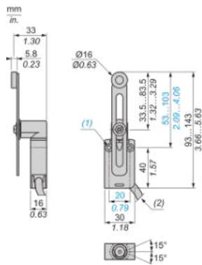
(1) 2 fixing holes Ø 4.2 mm, counterbored Ø 8 mm by 4 mm deep.
