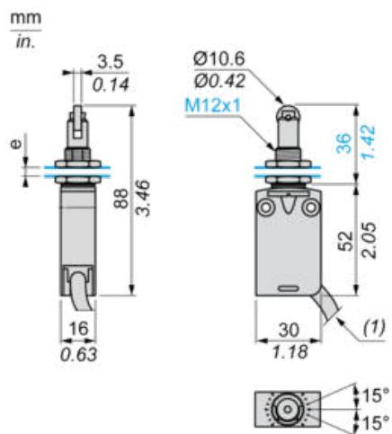
(1) External diameter of cable 7.5 mm.
