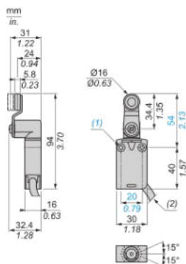
(1) 2 fixing holes Ø 4.2 mm, counterbored Ø 8 mm by 4 mm deep.
