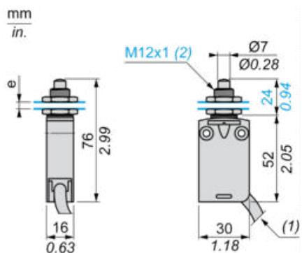
(1) External diameter of cable 7.5 mm.
