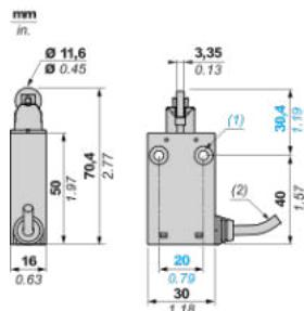
(1) 2 fixing holes Ø 4.2 mm (0.16 in.), counterbored Ø 8 mm by 4 mm deep (counterbored Ø 0.32 in. by 0.16 in. deep).
