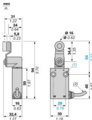
(1) 2 fixing holes Ø 4.2 mm (0.16 in.), counterbored Ø 8 mm by 4 mm deep (counterbored Ø 0.32 in. by 0.16 in. deep).
