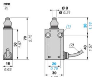
(1) 2 fixing holes Ø 4.2 mm (0.16 in.), counterbored Ø 8 mm by 4 mm deep (counterbored Ø 0.32 in. by 0.16 in. deep).
