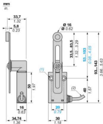
(1) 2 fixing holes Ø 4.2 mm (0.16 in.), counterbored Ø 8 mm by 4 mm deep (counterbored Ø 0.32 in. by 0.16 in. deep).
