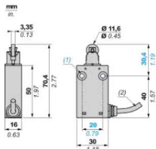
(1) 2 fixing holes Ø 4.2 mm (0.16 in.), counterbored Ø 8 mm by 4 mm deep (counterbored Ø 0.32 in. by 0.16 in. deep).
