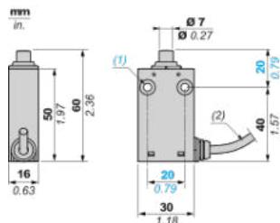
(1) 2 fixing holes Ø 4.2 mm (0.16 in.), counterbored Ø 8 mm by 4 mm deep (counterbored Ø 0.32 in. by 0.16 in. deep).
