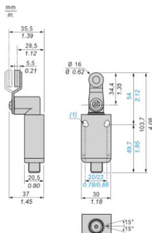
(1) : 2 elongated holes Ø 4.3 x 6.3 mm on 22 mm centers or 2 holes Ø 4.3 on 20 mm centers.
