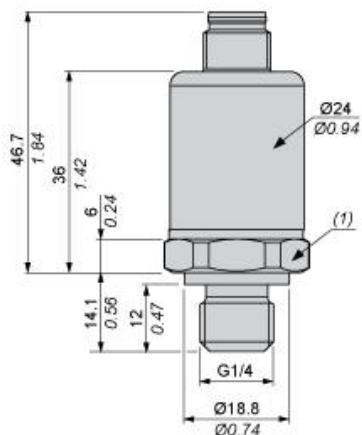
(1) SW24, tightening torque  24 N·m / 212 lb-in
