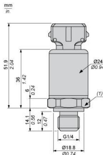
(1) SW24, tightening torque □ 24 N·m / 212 lb-in
