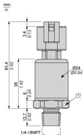
(1) SW24, tightening torque  24 N·m / 212 lb-in
