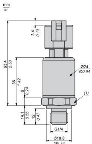
(1) SW24, tightening torque □ 24 N·m / 212 lb-in
